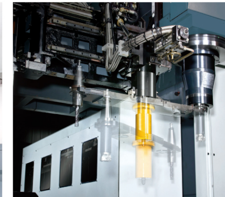
Extended head exchange on vertical type(opt.)
