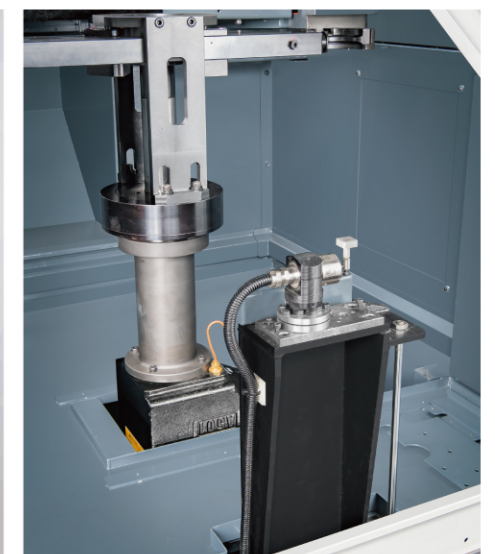
Contact automatic tool length measurement
