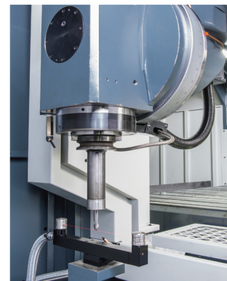
Non-contact automatic tool length measurement
