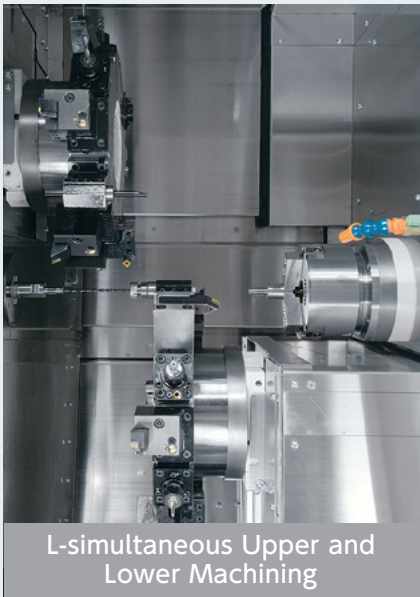
Upper turret on L-spindle / Lower turret on R-spindle
