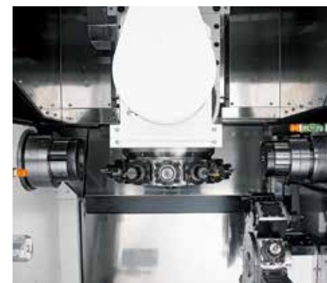
Upper left side, lower right side milling
